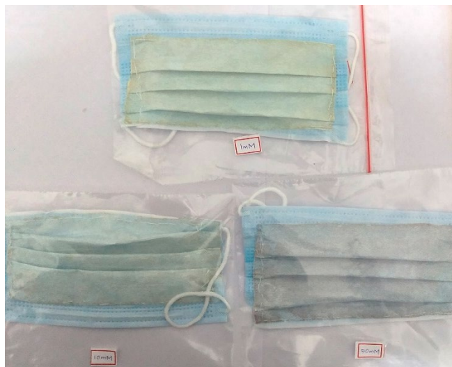
Masks developed using coated PP layer
